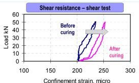
Increase of confinement is observed at early stage, larger contact area between crack surfaces is expected.
