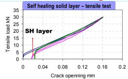
Thickness of SH layer after curing is around 10µm in each surface. Solid layer is overlapped by new layer by further curing.
