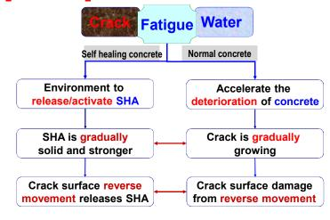
Self healing technology may improve the performance of concrete subjected to Seismic Loading
